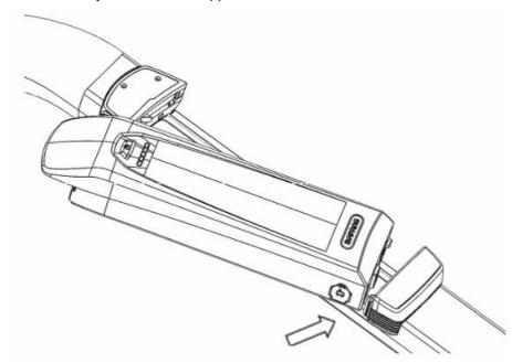
2. Push the battery into the battery holder, when hears a 'click' sound, that means battery is locked.
