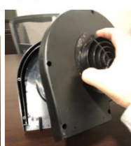
Mount bottom of housing and fasten with the 5 provided screws
