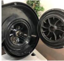
Mount fan onto arbor with the top (hex pocket) up. Align with hex on arbor. Fan will be flush to top of housing by spin freely.
