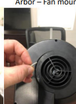
Mount bottom of housing and fasten with the 5 provided screws
