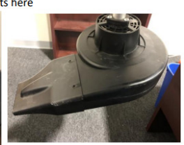
Slide nozzle on and fasten with screws provided.
