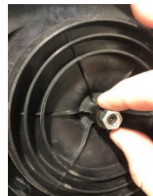
Put on Washer, lock washer and nut. Use pliers or wrench to tighten nut. Just hold the fan to snug up the nut.
