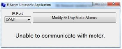
Make sure you have correctly installed the IR reader and selected the COM port to which it is connected. **NOTE:** Alarm modification does not work in high resolution meters. If you try alarm modification on a high resolution meter, you will see this message.
