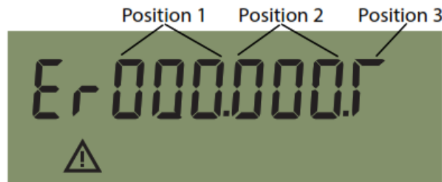
Figure 10: Alarm and operating mode screen in transition mode
