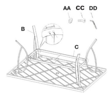
• Step 2: Attach the leg brace (C) to each leg (B). Use the hex key (DD) to tighten the short bolts (CC). you can tighten the all bolts now.
