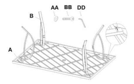
• Step 1: Place the contents on a soft, flat surface. Align the leg (B) to the table top (A) as shown in the image above. Use the hex key (DD) to tighten the long bolts (BB), being careful not to overtighten.
