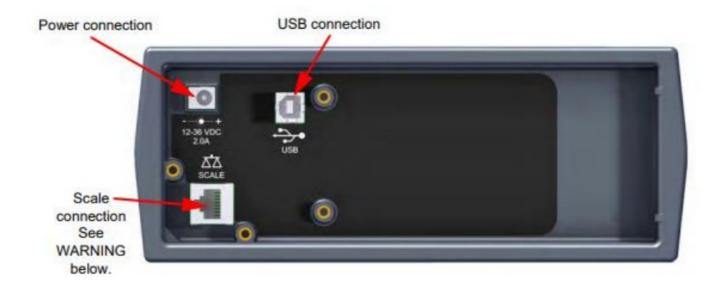
**WARNING:** The scale connection is an RS232 port only, Do not plug the base into an Ethernet port as this may damage file Ethernet hub.
