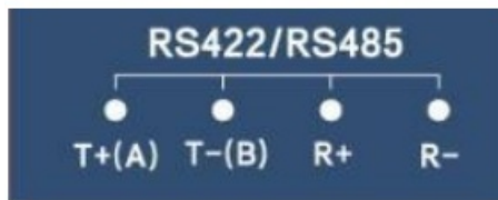
Figure 5 RS422/RS485 pin definition
