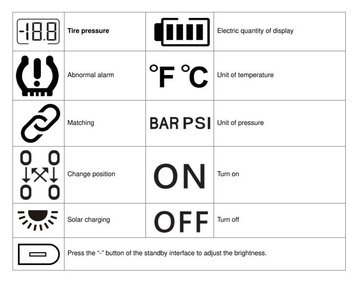
Caution: Turn on the power of the display and then install the sensor. Follow this step, and the data can be displayed at real time.
