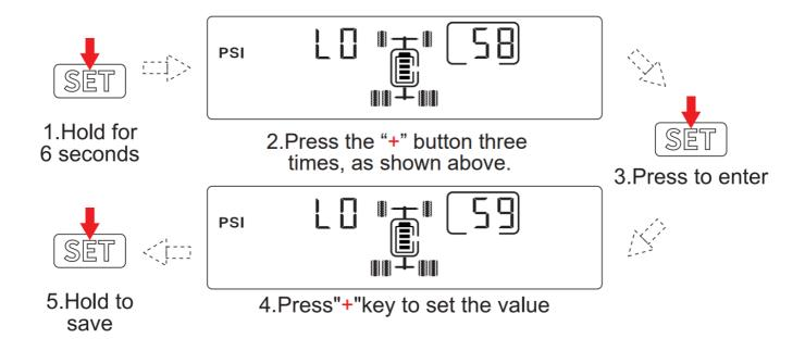
Setting of upper alarm value of Second axle tire pressure
