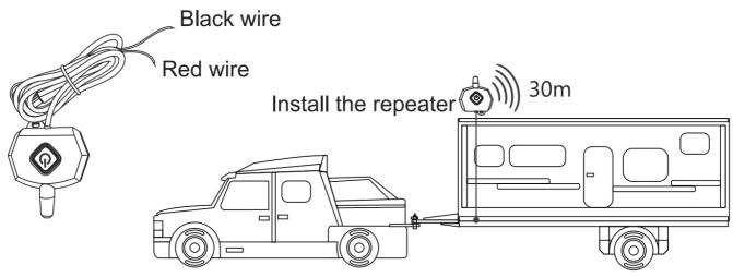
Repeater can make sure to strengthen the signal within 30m.Red cable connects with the anode of the battery. and the black cable connects with the cathode. The button on repeater flash with red light means ii is working normally. Otherwise, you need to confirm whether the repeater is properly connected. Or it may be broken if still not flash.
