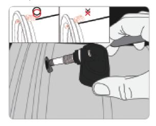
2. Install the washer first, and then use the wrench to install the nut. After pumping up, close the nut and install it.
