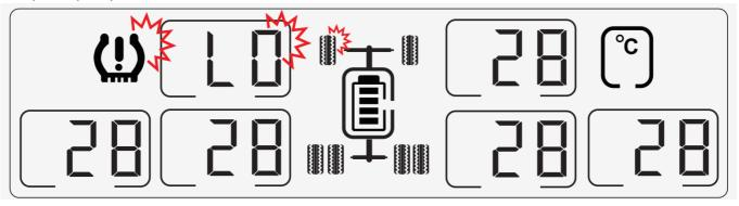
After the display alarms, press anywhere on the display to remove the prompt sound, and the flickering prompt will continue till the fault is removed
