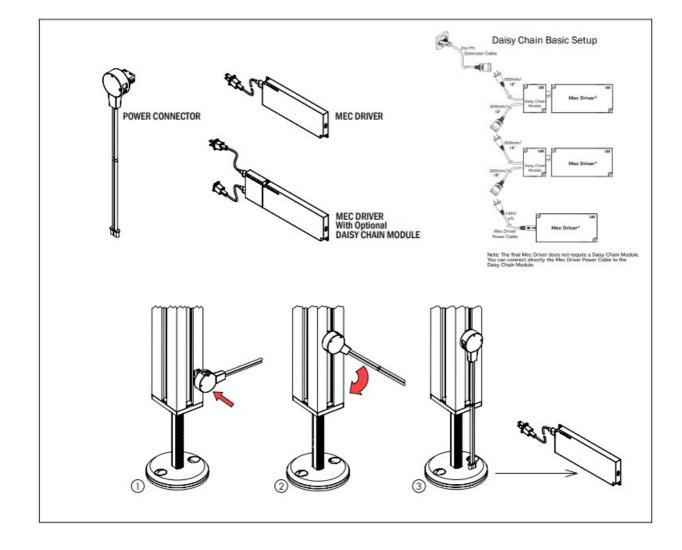
**GENERAL SCOPE**: Power is supplied to the Sorbetti Upright by means of a Power Connector attached to a driver. The Power Connector can be attached to any of the four sides of the upright and anywhere along the vertical. It is recommended to be attached in the most inconspicuous spot available with easiest access for the driver and power outlet.
