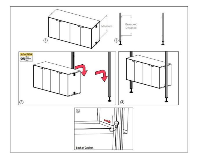
**GENERAL SCOPE:** Installing the larger cabinets requires a slightly different approach than installing smaller accessories. It is recommended the install is done with two people lifting. Also these wooden cabinets use two Pole Plates per side.
