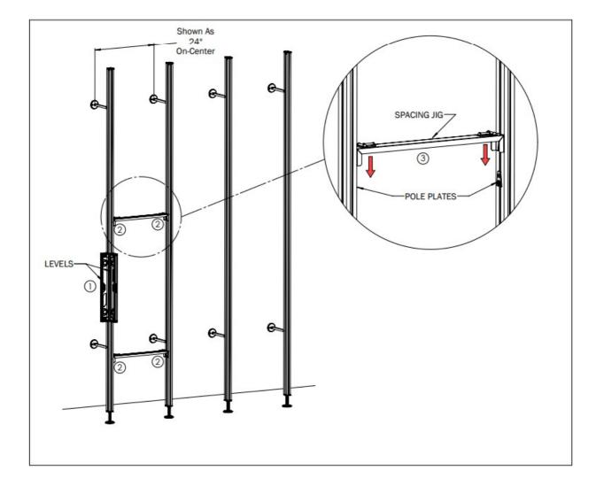
**GENERAL SCOPE:** After installing the first upright, additional uprights can be installed easily with the aid of the Spacing Jig.
