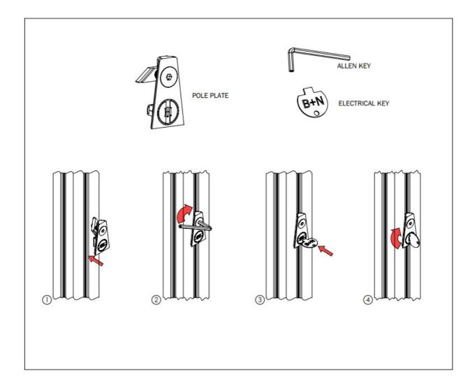
**GENERAL SCOPE:** Pole Plates serve two purposes. The first is to support the accessory. It does so using a locking taper, which creates an incredibly strong and rigid connection. The second purpose of the Pole Plate is to deliver power to the accessory. Pole Plates can be installed on any of the 4 surfaces of the upright, at any location on the vertical.
