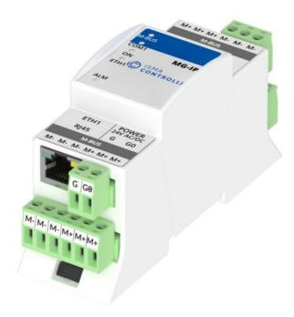
Meter Gateway with built-in M-Bus to M-Bus IP gateway with power supply for up to 60 devices and Modbus TCP/IP to Modbus RTU Gateway.
