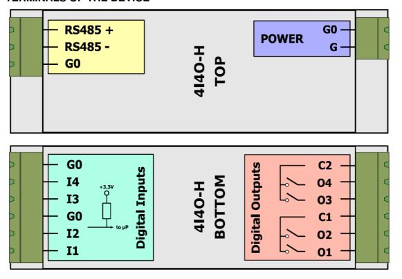
All G0 terminals are connected together internally
