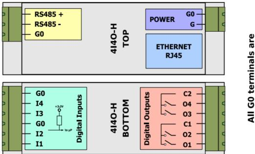
All G0 terminals are connected together internally
