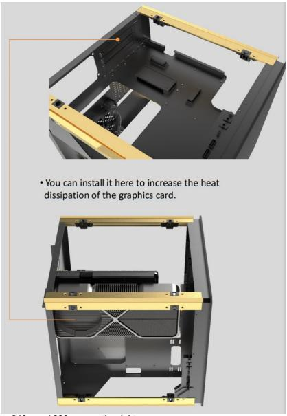
5. Supports radiators up 240 mm / 280 mm on the right Supports radiators up 240 mm / 280 mm on the left
