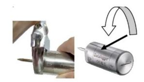
3. Remove the old battery and O-ring and install the new batteries. Pay attention to the polarity of the battery.
