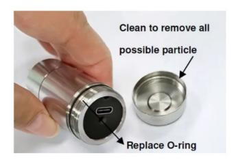
To close, turn clockwise to match the alignment mark.
