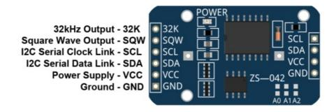
The DS3231 RTC module safely operates in 3.3V Voltage.
