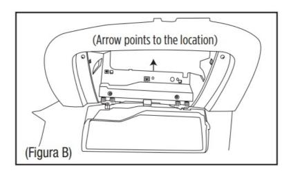
• This module is located behind the glove box. There are (2) modules behind the glove box. This module is behind the metal dashboard support. (Figura B)
