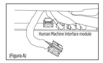
• Connect the female 12-pin harness with a Yellow RCA jack, to the male Gray harness removed from the Human Machine Interface module. (Figura A)
