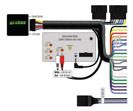
3.5mm Adapter (for radios witha wireforSWC)
