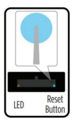
1. If the interface fails to function, press and release the reset button, then repeat the programming process from step 4 to try again.
