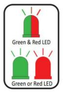
The LED will flash Green & Red while the interface programs the radio to the steering wheel controls. Once programmed, the LED will go out, then produce a pattern that will identify the radio type installed. Refer to the Radio LED Feedback section under Troubleshooting for radio types.
