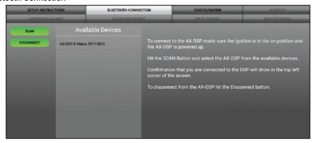
• **Scan** – Press this button to start the Bluetooth pairing process, then select the available device once it is found. "Connected" will appear in the top left corner of the app once paired.
