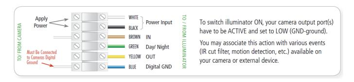
Make all electrical connections BEFORE applying power.
