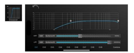
InIn this menu, you can assign a frequency band to the connected speakers that corresponds to their recommended frequency range. You can choose independent crossover settings for each channel individually or for all left and right channels together. Simply use the "Combine" button at the bottom right and choose whether you want to copy the values from the left channels to the right or from right to left.
