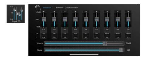
Depending on the source, it may be necessary to smooth the input signal to achieve a better input signal. This may be necessary for vehicles with a simple OE speaker system without separate tweeters. Some of the OE head units in these vehicles, for example, have an extremely high treble level to get more treble from the full-range speaker. You can set the input EQ for each source separately. You can adjust the input EQ for each source separately.
