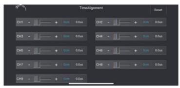
In this menu, you can apply a delay to the speaker signal to simulate an ideal listening position. Here's how to do it: Note the distance between your listening position and the individual speakers. Select the farthest speaker as the reference for the other speakers. Use the following example to calculate the values for your speakers:
