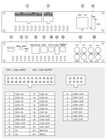
REM-Out: Connect this wire to the remote input of a separate amplifier, for example a mono amp for a subwoofer. It provides max 0.3 A.
