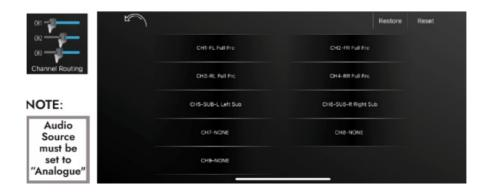
In this menu, you can assign an input signal to each output channel, including the desired gain level. It is also possible to combine two or more input signals into one output channel. For better clarity, you can also name each channel
