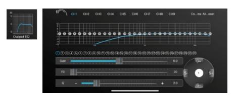
You can create your sound according to your settings in the EQ menu. Depending on the grade of required accuracy, you can adjust up to 31 bands of the parametric equalizer.
