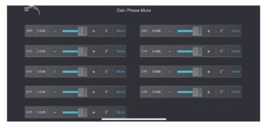
In this menu, you can make the following settings for each individual channel: volume, mute, and phase. Adjust the gain using the slider or the +/- buttons. Tap on 0 degrees in the second-to-last column to switch between 0 degrees phase or 180 degrees phase (reversed electrical phase). Tap on Mute to mute or unmute the channel. The settings for Gain/Phase/Mute also apply to the corresponding preamp outputs.
