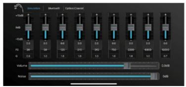
Depending on the source, it may be necessary to smooth the input signal to achieve a better input signal. This may be necessary for vehicles with a simple OE speaker system without separate tweeters. Some of the OE head units in these vehicles, for example, have an extremely high treble level to get more treble from the full-range speaker. You can set the input EQ for each source separately. You can adjust the input EQ for each source separately.
