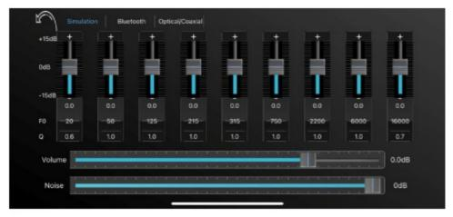
Depending on the source it might be necessary to flatten the input signal to receive an accurate sound signal. This could be necessary especially in cars with basic OE speaker system without separate tweeters. Some of the OE headhunts of those cars are provided with an extreme treble volume to get more treble sound out of the broadband speaker. You can adjust the input EQ for each source separately. You can adjust the Gain from -15 dB to + 15 dB
