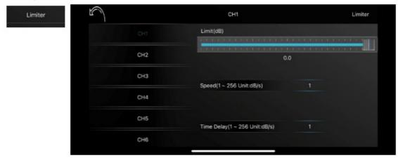
The limiter function is the reinsurance if you drive your car stereo hard on the limit. Turn up the volume until you listen to distortion of the sound, especially the woofers and subwoofers. Now choose the limit (db) value how much the limiter should reduce the sound volume level, choose the speed how quickly the limiter shall reduce the sound volume level and finally how long the limiter shall reduce the sound volume level.
