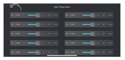
In this menu you can adjust the following settings for each individual channel: sound level, mute and phase. Adjust the gain by using the slider or with the +/- buttons.
