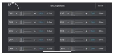
In this menu you can apply a time delay to the speaker signal to simulate an ideal listening position. How to do:
