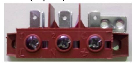
The device must be connected directly to the mains and must have an easily accessible switch from the start stalled for the device according to the national, international and local laws in the country where it is installed. This switch must separate polarization guaranteeing complete disconnection in accordance with the overvoltage III category.
