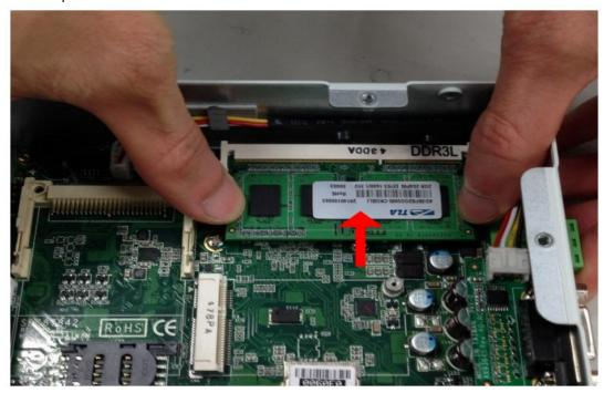
**Step 4** The memory module is locked by two latches on the sides. We strongly recommend using "LDC737" silicone on the two sides of the memory for good ability of vibration.
