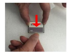
Step 4 Insert the CF card into the socket tightly and lock the CF card.
