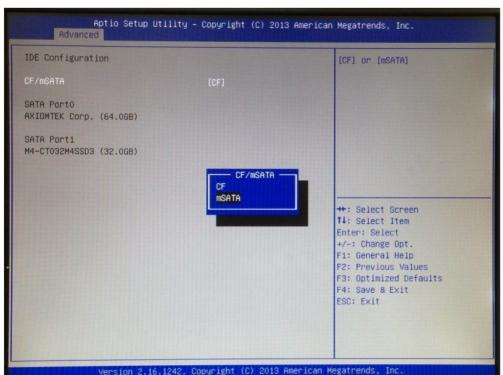
Note: CF and mSATA function can be either one, it can be select by BIOS menu. mSATA and wireless use the same slot, and only one of them can be selected
