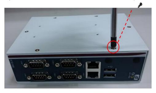
Step 3 Loosen 4pcs screws of the cover, and put the HDD into the HDD bracket and fix the HDD by 4pcs of
