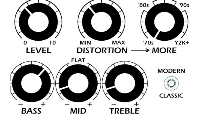
**LEVEL:** Increases the output volume level as the knob is turned clockwise.
