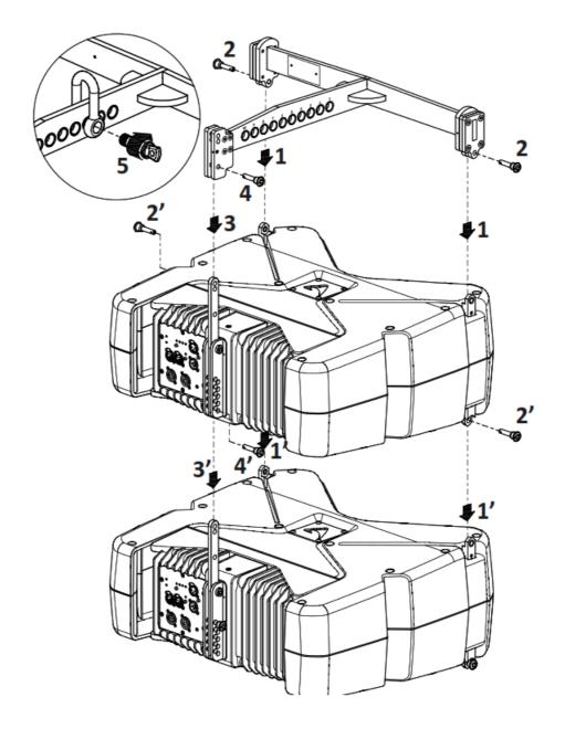
**KPTAX800L** fly bar maximum capacity is 680 Kg (1500 lbs) with the  $0^{\circ}$  angle. It can support, with a safety factor of 10:1, up to:
