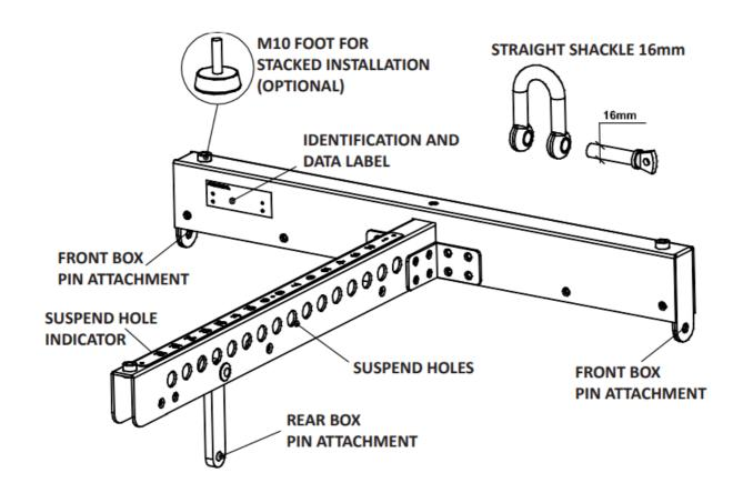
**WARNING:** KPTAX2012P fly bar maximum capacity is 700 Kg (1540 lbs) with a 0° angle. It can support up to 12 AX2010 loudspeakers with a safety factor of 10:1.
