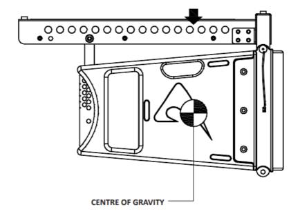
The figures below show how to insert correctly the locking pin, always carefully check that each pin is fully inserted and locked in the correct position. Set up the splay angle between loudspeakers inserting the pin in the correct hole, please note that the inner hole in the hinge top is for whole angles (1, 2, 3 etc.) while the outer hole is for the half angles (0.5, 1.5, 2.5 etc.).
