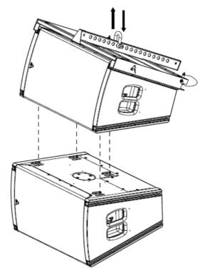
4. Link the first box to the second box using two coupling bars: remove the pins and the locking plates and insert the bars into the cabinet rails from the front.
