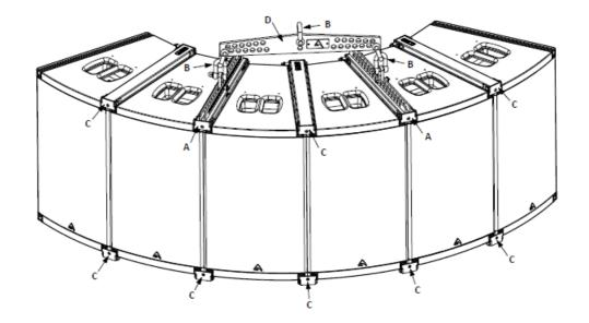
For horizontal arrays made of more than 6 loudspeakers, as a rule of thumb, one KPTAX1012H flying bar should be used at most every two or three boxes, as in the following examples. When flying arrays with more than 6 units, it is advisable to use multiple lifting points connected directly to the KPTAX1012H flying bars, without using the KPTAX1012T suspension bars.
