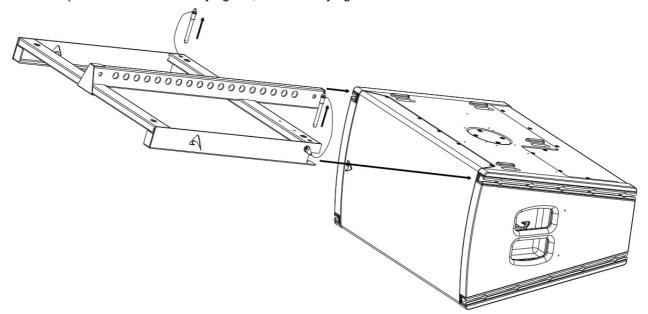
2. Put back in place the pins in their hole, making sure that they are inserted correctly. Fix the shackle in the chosen hole and link the lifting system.
