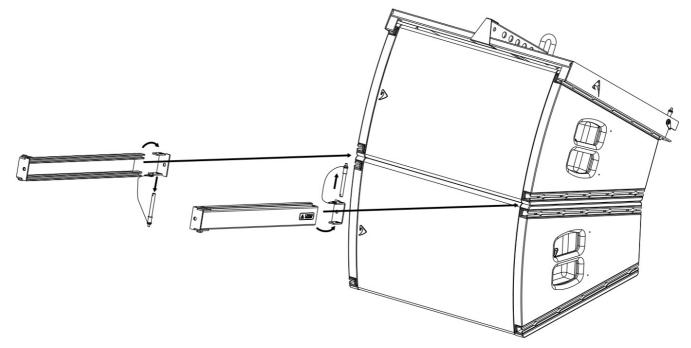
5. Put back in place the locking plates and fix them reinserting the pins in their hole.
