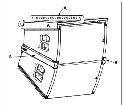
3x AX1012A VER. ARRAY 100° x 60° coverage 114.5 Kg total weight list of rigging material: A) 1x KPTAX1012V B) 4x KPTAX1012
