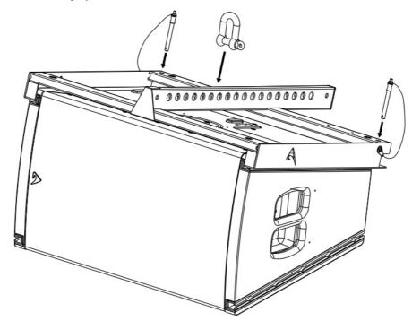
3. Lift the first box, place the second box on the floor just underneath the first one. Let down slowly the first box
