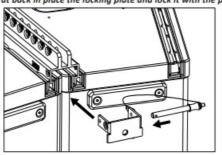
5) Place the cam into the hole chosen for lifting: always be sure that all pins are firmly inserted in their position.
