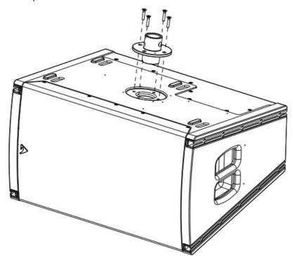
3. Insert the KP010 tilt adapter into the KPAX265 and install the AX1012A to the pole. Aim the tilt adapter 10° down to align the AX1012A to the floor and fix its pin. Adjust the pole's height if needed.
