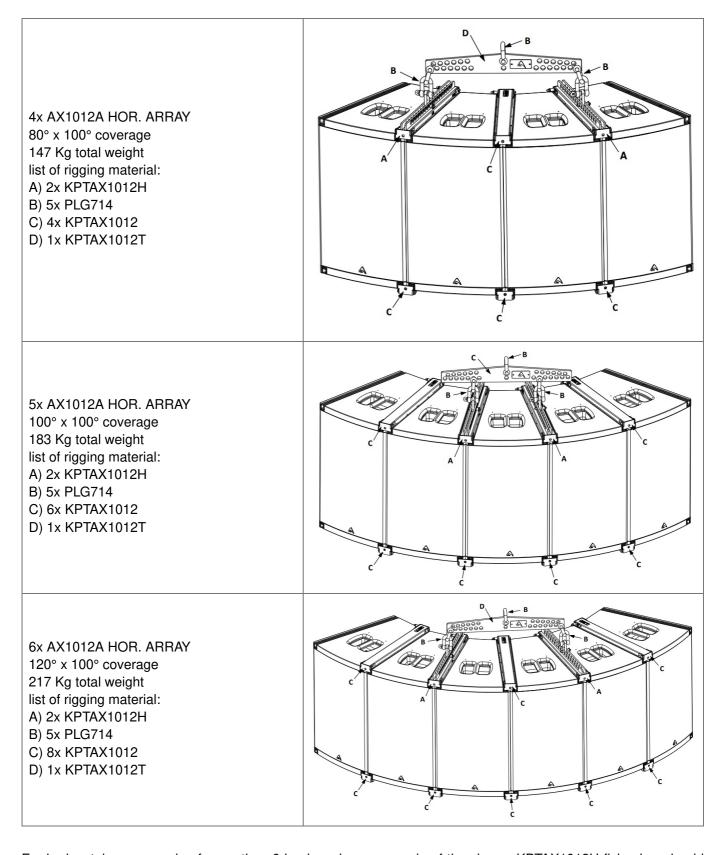
For horizontal arrays made of more than 6 loudspeakers, as a rule of thumb one KPTAX1012H flying bar should be used at most every two or three boxes, as in the following examples. When flying arrays with more than 6 units, it is advisable to use multiple
