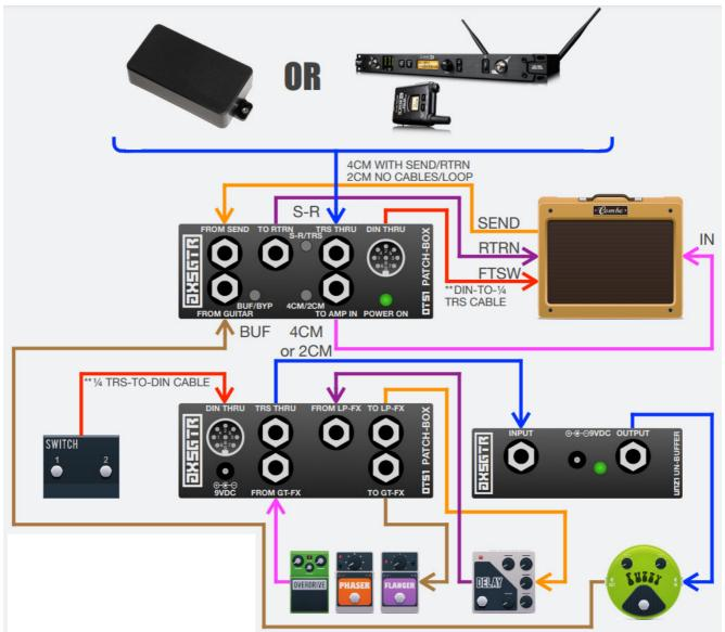
Press the OTS1 Patch-Box 4CM/2CM button to instantly reconfigure the pedalboard signal path when using an amplifier with an effects loop, the 4CM Pl. or one without, the 2CM /OUT].
