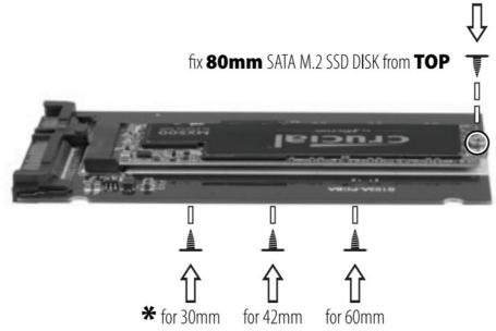
$^{\star}$  fix 30mm, 42mm, 60mm SATA M.2 SSD D I S K w i t h nut fom BOTTOM
