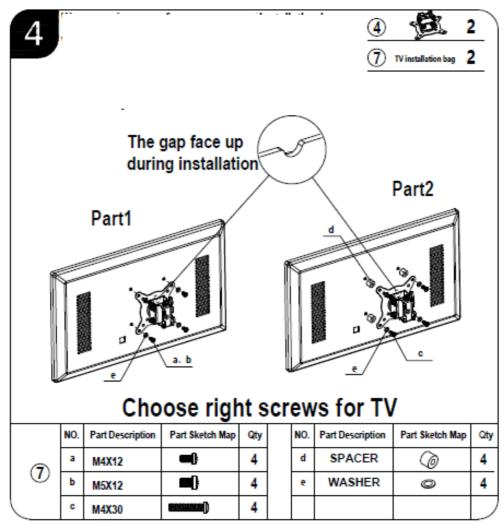
5. See the picture ,first put into the groove of part no post then fasten down.
