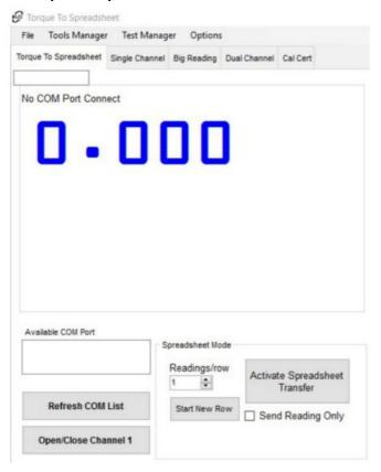
This module allows the user to export the reading from testers directly into an Excel file (works as a terminal emulator). Click on "Activate Spreadsheet Mode." Open an excel file and place mouse cursor on any cell of Excel Spreadsheet. Each reading will be exported into the Excel file where the cursor is located.
