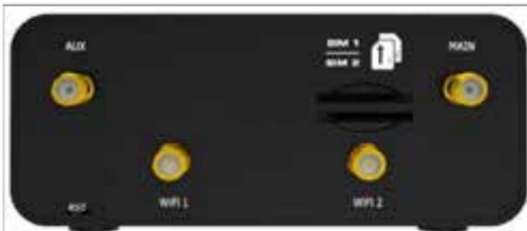
**Please Note:** Your AMR984X will function fully with only one SIM, which can be inserted into either slot.
