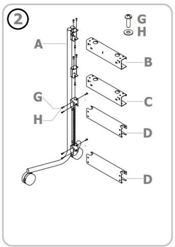
Attach the other Leg (A) to the Horizontal Supports (B) (C) (D) using the Bolts (G) and Washers (H) as shown.
