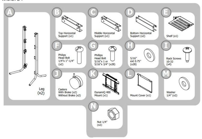
**Install Tip:** As you are installing the bolts and nuts, leave them all loose. Install all of them before tightening. Attach Casters (J) to the end of each Leg (A). Make sure the Casters with Brakes are installed in the front of the cart.
