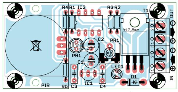
Figure 2. Arrangement of components on the PCB
