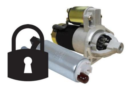
This unit is a 2-point immobiliser, meaning relays can cut off both the starter motor and fuel pump, providing a two-pronged method of vehicle immobilisation
