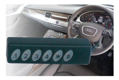
If the unique 4-digit code is not entered correctly up to 15 seconds before ignition, the vehicle will not be functional. To deter code guessing, the keypad locks for one minute after 3 incorrect attempts.
