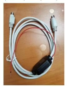
**Note**: The red power cord is connected to the radio +13.8V power supply. In February 2023, manual accessories 6-pin thread enhanced version, tentative number: 6P-10P conversion board, 6P-10P conversion board series accessories 6P-6P- plus cable. Including but not limited to the following models for connection use:
