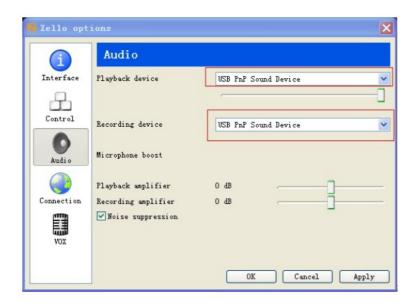
set the audio on both input and output to USB PnP Sound Device (windows the operating system already has
