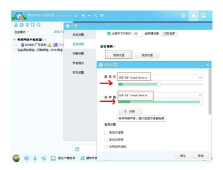
On the YY channel, select both the microphone input and speaker output to "USB PnP Sound Device" on the system audio management interface, please do not select microphone enhancement or AGC, if you select the option, the audio of the other party will be very loud and noisy
