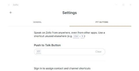
**Note:** The new version of ZELLO does not support the middle mouse button mode, you need to run "MouseChange". Convert the "middle mouse button" to the keyboard value "F7". The window is minimized to run. At this time, R1 internal detection will be converted to "F" 7 to trigger ZELLO forwarding. Program MouseChange download website: <a href="avrtx.cn">avrtx.cn</a>
