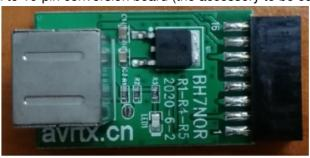
The above 6-pin to 16-pin conversion board, it is for Motorola radio and is to use for connection on GM300 SM50 SM120 GM338 GM339 GM398 GM3188 GM3688 GM950I CDM-1250 GM140 GM160 GM340 GM360 GM380 GM640 GM660 GM1280
