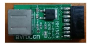
The above 6-pin to 16-pin conversion board, it is for Motorola radio and to use for connection on GM300 SM50 SM120 GM338 GM339 GM398 GM3188 GM3688 GM950I CDM-1250 GM140 GM160 GM340 GM360 GM380 GM640 GM660 GM1280
