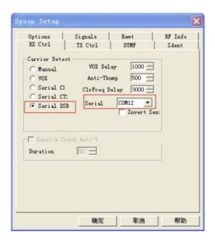
Set receive control as: Serial DSR Select: USB serial number
