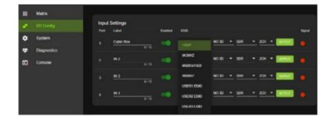
Input Settings Label – This is where inputs are given a name/alias (Apple TV, Cable Box, Roku, etc.). Note: There is a 15-character limit to this field; the name will replace the default IN # throughout the rest of the WebUI (for instance, the Video Matrix tab)
