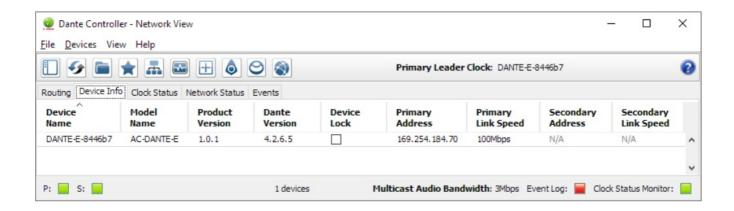
**Note:The** computer running Dante<sup>™</sup> Controller and the AC-DANTE-E must both have a physical connection to the Dante<sup>™</sup> network in order for the AC-DANTE-E to be discovered by Dante<sup>™</sup> Controller.
