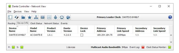
The computer running Dante™ Controller and the AC-DANTE-E must both have a physical connection to the Dante™ network in order for the AC-DANTE-E to be discovered by Dante™ Controller.
