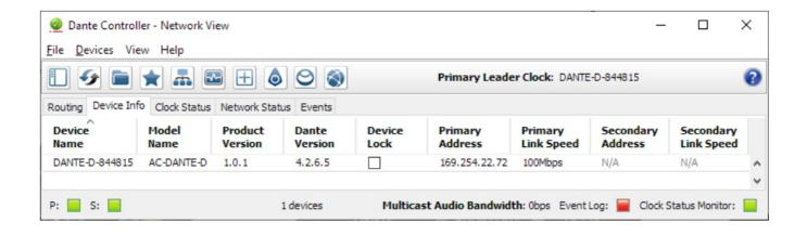
**Note:** The computer running Dante<sup>™</sup> Controller and the AC-DANTE-D must both have a physical connection to the Dante<sup>™</sup> network in order for the AC-DANTE-D to be discovered by Dante<sup>™</sup> Controller.
