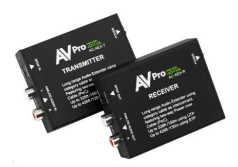
The AC-AEX-KIT is a basic solution for extending audio signals up to multichannel 5.1. It comes with Bidirectional POC (Power over Cable) and can send both analog and digital signals up to 100 meters over traditional Cat5e and up to 130 meters over shielded Cat5e. The AEX has a Dual Play function, allowing simultaneous playback on both the analog and digital output, regardless of input.
