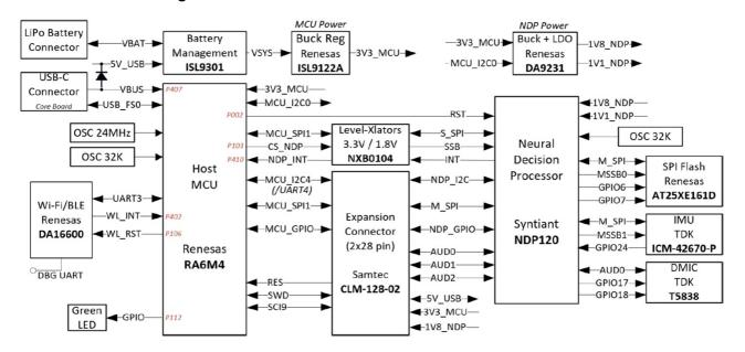
RASynBoard Starter Kit adds an IO Board (50mm x 30mm), for a versatile, compact, two-board evaluation kit assembly. This pins-out a subset of the NDP120 and RA6M4 I/Os to popular Pmod, Click header and expansion header footprints, enabling connection with additional external microphones and sensor options. An onboard debugger MCU (SWD and UART interfaces), button switches, RGB LED and removable MicroSD storage, further maximize the prototyping versatility and utility.
