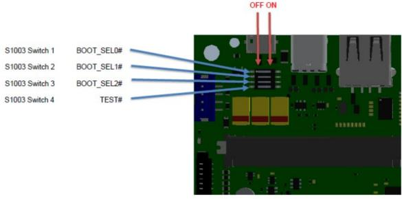
The following table describes the available boot options for the Edge Al Kit. See the i.MX 8M Plus Applications Processor Reference Manual from NXP for a complete description.
