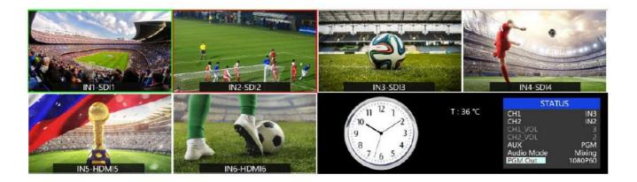
The lower right corner display of the menu and status information. The CH1, CH2 are the channel selection of the 2 audio sources for audio mixer. There is a real-time Digital clock/Analog clock displayed beside the menu.
