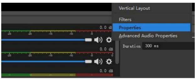
**Step4.** Enter "Advanced Audio properties" can change the setting about the volume, balance, audio monito ring, and Tracks etc.
