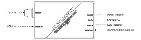
**Note:** When both SDI and HDMI are plugged, SDI input signal will take priority. When both SDI/ HDMI IN and **AUDIO IN** are plugged, external audio input will take priority.
